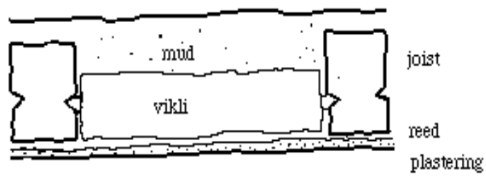
section of ceiling over first kitchen and verandah
